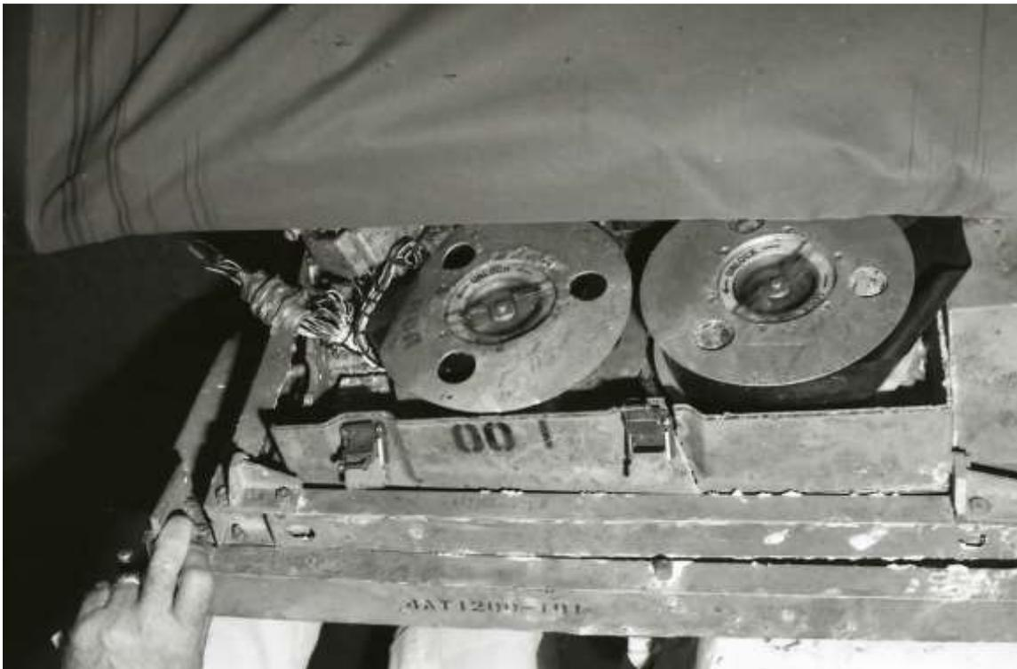
**Ampex recorder/playback machine for recording ELINT and Nav data.**
